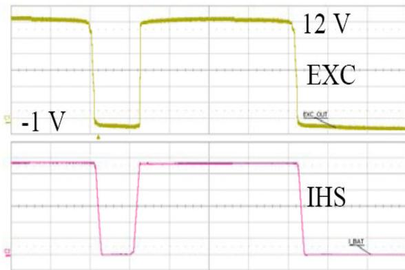
Alternator demonstrator switching
