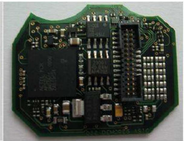
brushholder for alternator demonstrator with flexible FPGA control
